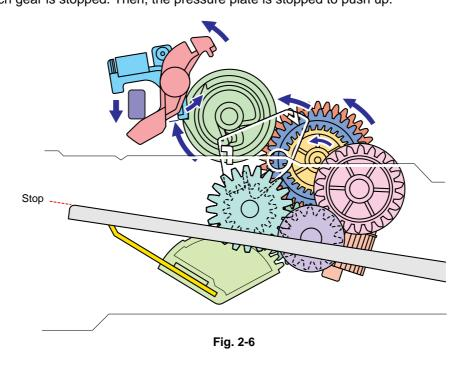
When the tray is pulled out from the printer, the pressure plate is returned to the original position. When the tray is put into the printer, the above operation is performed from the start again.
