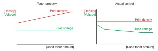
To obtain a print result of a constant density all the time, the printer counts the number of print pages immediately after the toner cartridge is replaced and changes the bias voltage according to the accumulated number of prints with the toner cartridge.
