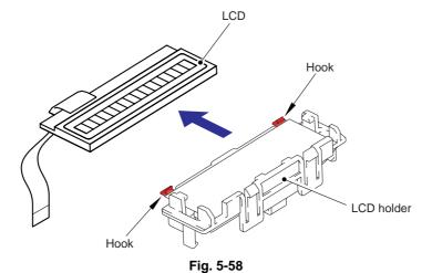
(4) Remove the Back light film from the LCD holder.
