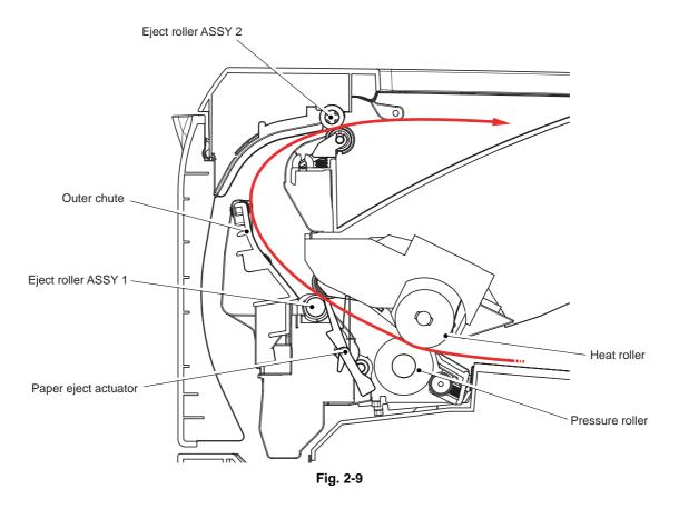
When a paper jam occurs, the main motor rotates conversely to throw out the engagement of the gear. Consequently, the eject roller ASSY 2 is released so that the jammed recording paper is removed easily.
