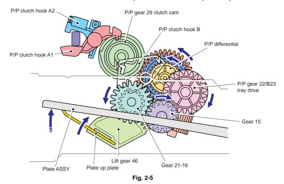
When the feed roller is pushed up, the hook is released by the lift arm, and the rotation of the clutch gear is stopped. Then, the pressure plate is stopped to push up.
