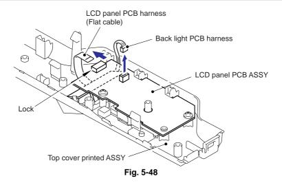
(3) Remove the three cup B M3x8 Taptite screws, and then remove the LCD panel PCB ASSY.
