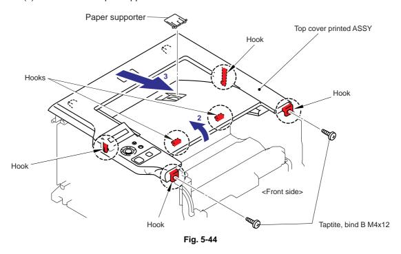
(5) Remove the Panel Plate Printed ASSY from the Top cover printed ASSY.
