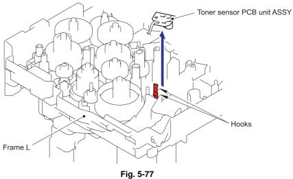
(2) Remove the PT sensor holder from the Toner sensor PCB ASSY.
